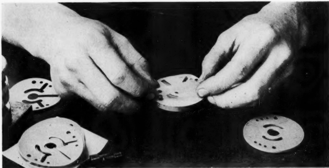
ASSEMBLY IS EASY: First step is to place the aluminum die casting (milled face up) on locating pins.
